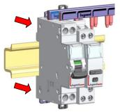
2. Unscrew the terminals and pull the device forward in order to release it from the DIN rail
