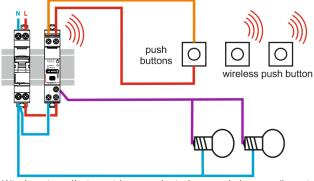
. Wireless installation with several wireless push-buttons " ... with Netatmo " controlling a connected latching relay (see page 6 for the association of wireless push-button) :
