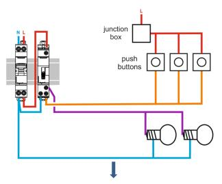
After: Installation « 3 wires » with line on the push-buttons
