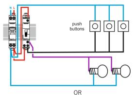
Installation « 4 wires » with line on the push-buttons
