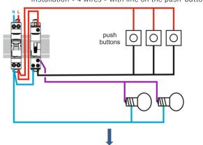
After: Installation « 4 wires » with line on the push-buttons
