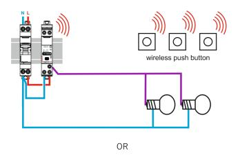
Installation « 4 wires » with line on the push-buttons
