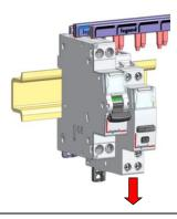
3. Pull the device downward in order to completely release it from the prongs of the busbar
