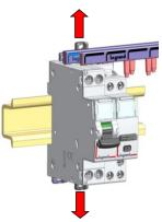
1. Unclip the clamp to put it in open position
